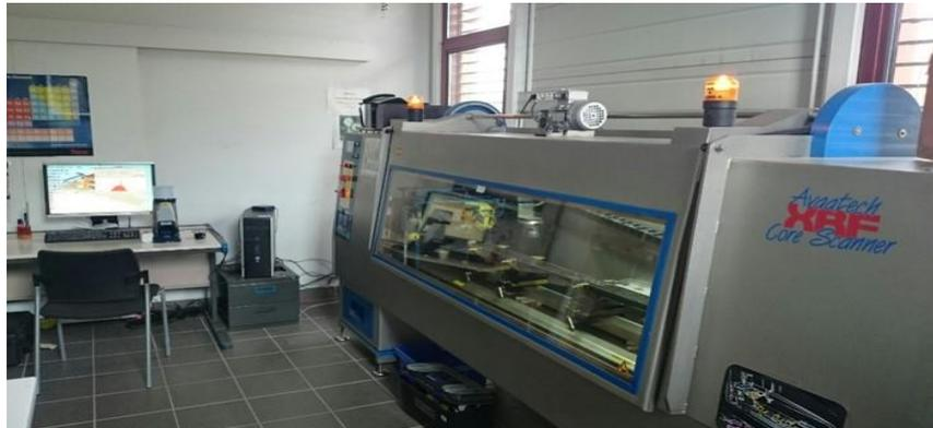
Core scanner XRF Energy Dispersive (CS-XRF-EDS) – Avaatech
